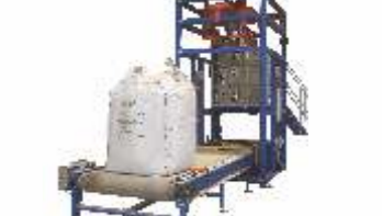
Out Feed Conveyor
